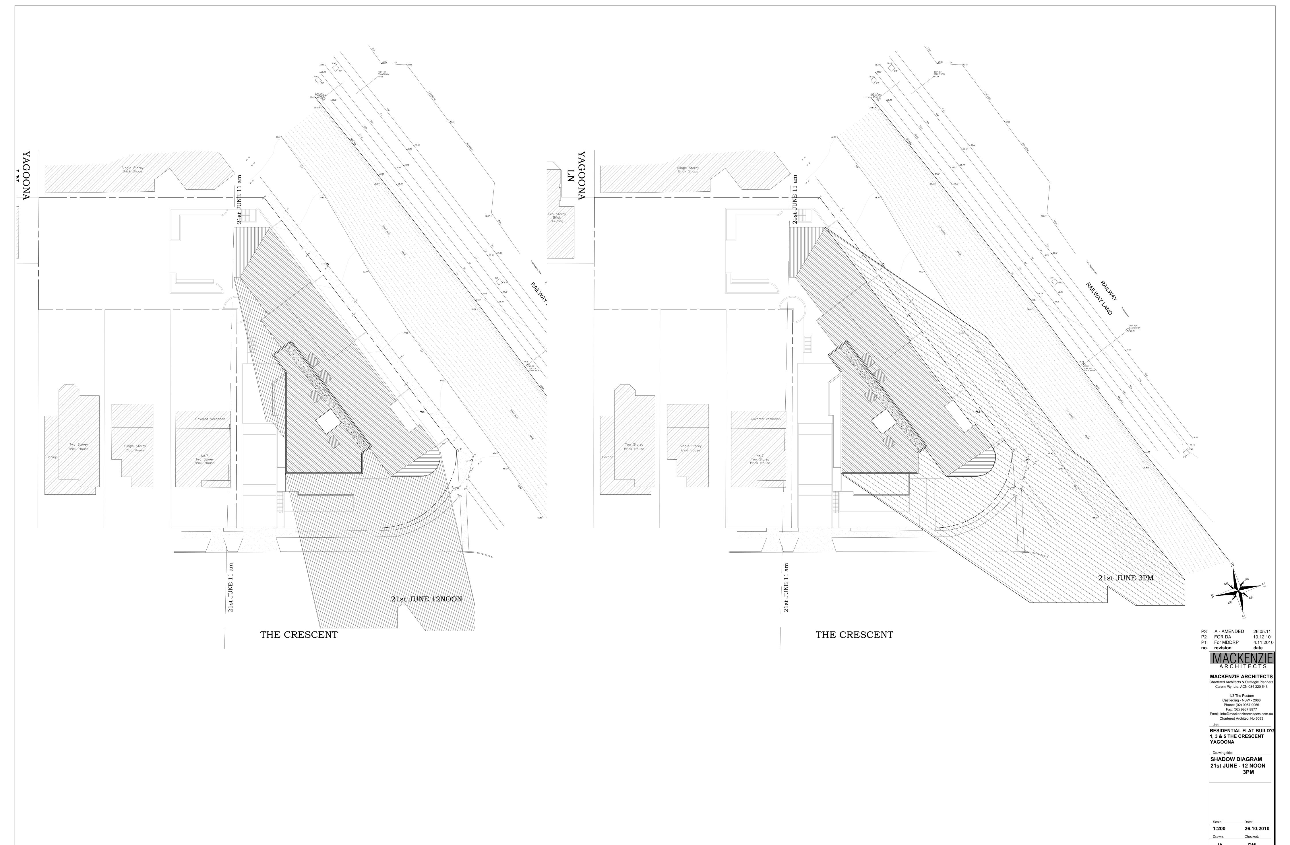
12NOON SHADOW DIAGRAM 21st JUNE SCALE 1:200 3PM SHADOW DIAGRAM 21st JUNE SCALE 1:200 Drawing no.
